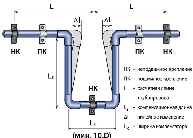
$$L_k = 2 \cdot \Delta I + 150 \text{ [мм]} \text{ при } L_k \geq 10.D$$
