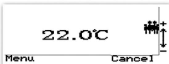
Pressing the PLUS or MINUS keys will allow you to change the set temperature up or down as shown in the examples below:
