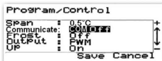
If COM Off is selected, no setback signal will be sent to the Slave thermostat. With COM 4C or COM 2C selected the slave thermostat temperature will be reduced or increased by 4 °C or 2 °C, depending on whether the system is in Heating or Cooling mode.
